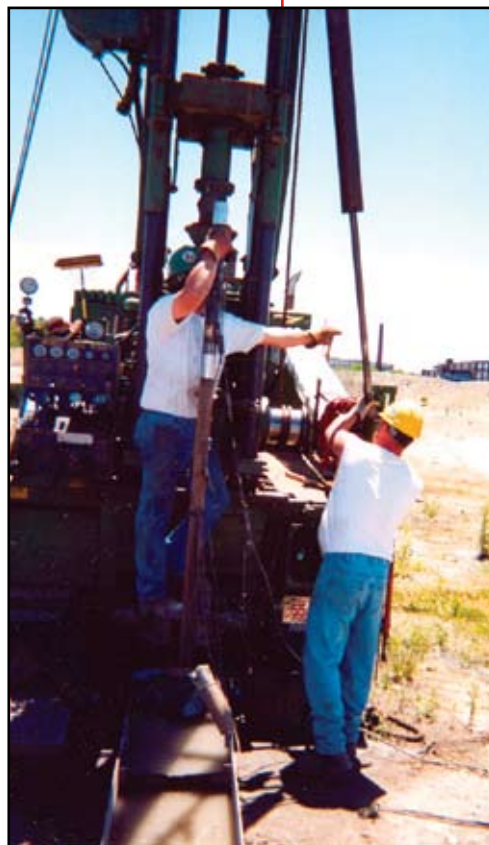
Attaching SPT to Instrumented Rod Section
