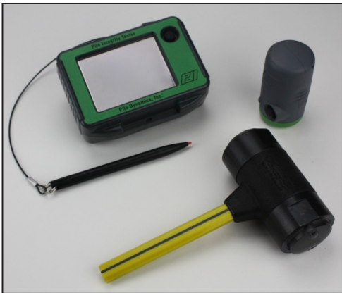
PIT-X with wireless accelerometer and handheld hammer.
