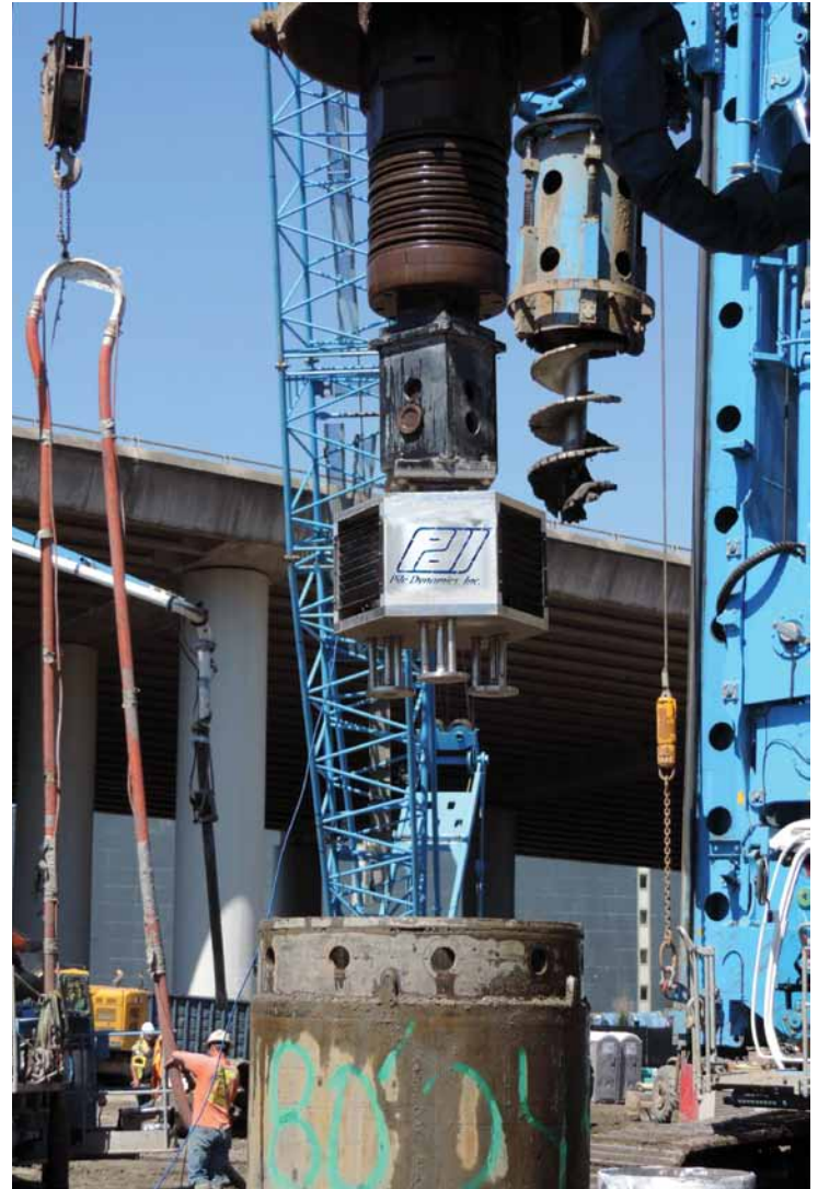
SQUID attached to Kelly bar, ready for test
